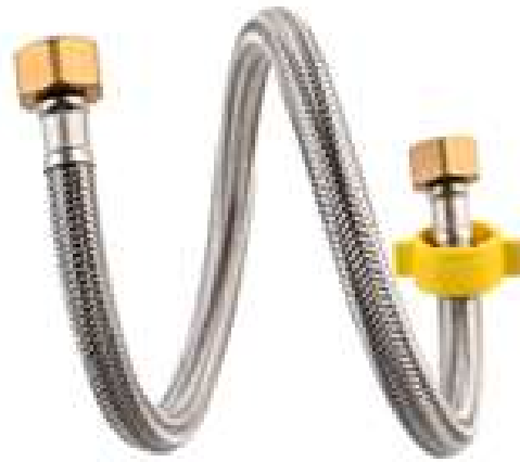
Braid hose BH002 S.S+Nylon braid hose Length: 50cm Brass nuts
